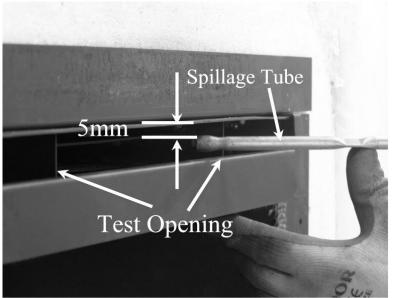
• If spillage is detected the cause must be discovered and the fault corrected, if the fault cannot be corrected, disconnect the fire from the gas supply and seek expert advice. Spillage can be caused by a restriction in the flue system, down draught or insufficient ventilation into the room where the fire is installed.
