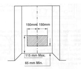
Drill holes for eye bolts on 112mm centre lines between maximum and minimum heights.
