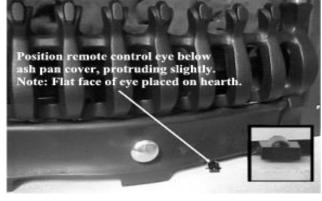
Check that a signal is being received by pointing the remote control hand set in the direction of the appliance and simultaneously press the buttons marked ' and 'standby'. Continue to hold in these two buttons until a 'bleep' is heard (approximately 2-3 sec.). If no sound is hear check position of remote control eye.
